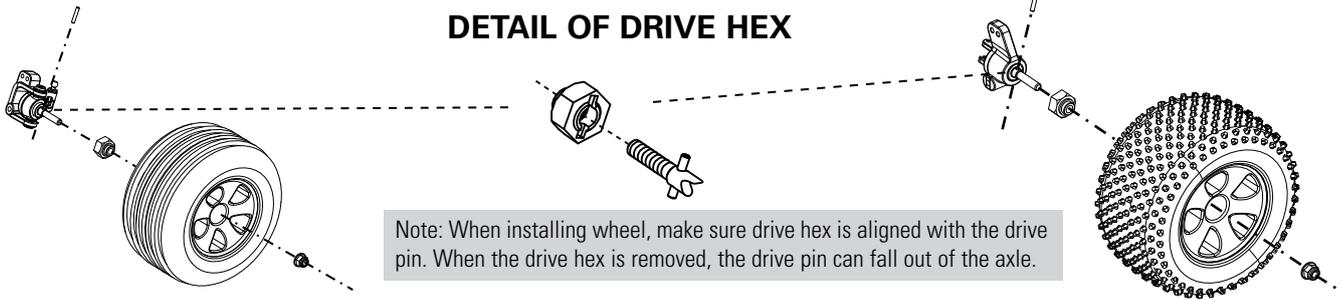
Note: When installing wheel, make sure drive hex is aligned with the drive pin. When the drive hex is removed, the drive pin can fall out of the axle.
